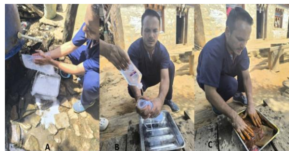
Figure 2: (A) Washing of PVC insect screen mesh using detergent and water; (B) rinsing with normal saline; (C) soaking in a povidone-iodine solution
